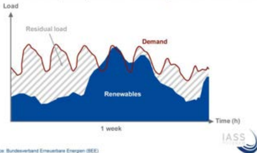
Figure 2: Residual load power plant fleet with a large share of renewables (Source: IASS based on data provided by the Bundesverband Erneuerbare Energien (BEE)). Source: Becker Report, p. 68.
